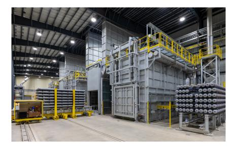
Hydro, a leading company in aluminium and renewable energy, relies on Hertwich Engineering's technology, a subsidiary of SMS group, for the construction of a recycling plant in Torija, near Spain's capital, Madrid. Hertwich's delivery includes three batch homogenization furnaces with two cooling chambers, a billet saw, an ultrasonic testing- and a packaging station. The new recycling plant is scheduled to begin operations in 2026.
