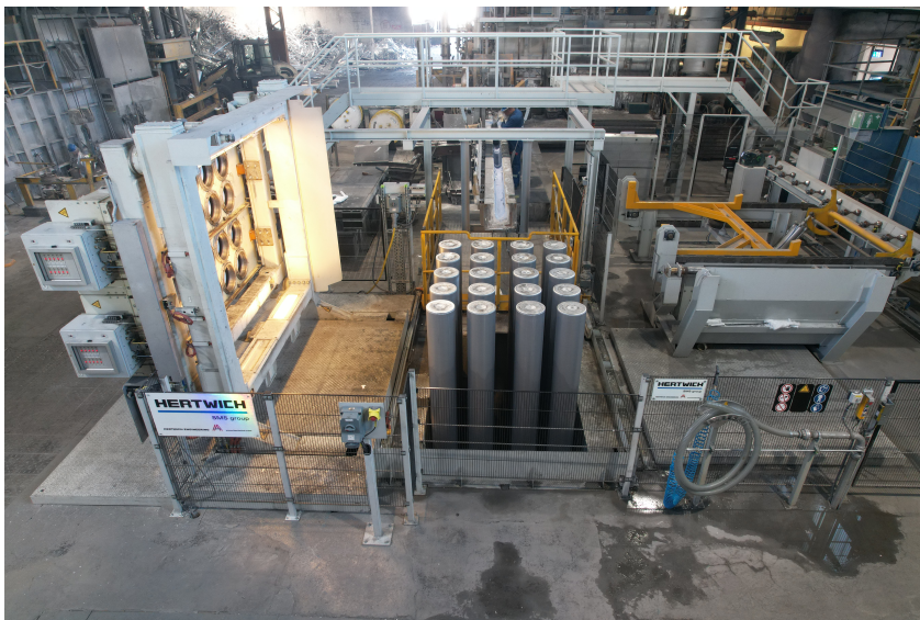
Hertwich VDC Vertical Direct Chill Caster
