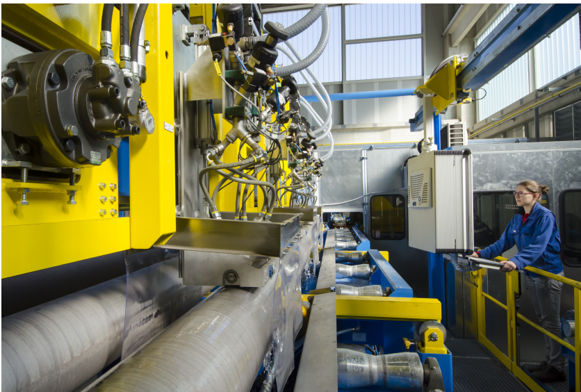
Helical Ultrasonic Testing Station at Impol d.o.o., Slovenia
