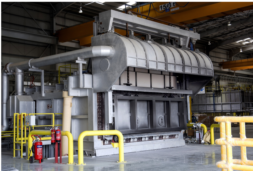
Casting Furnace, capacity 30 tonnes
