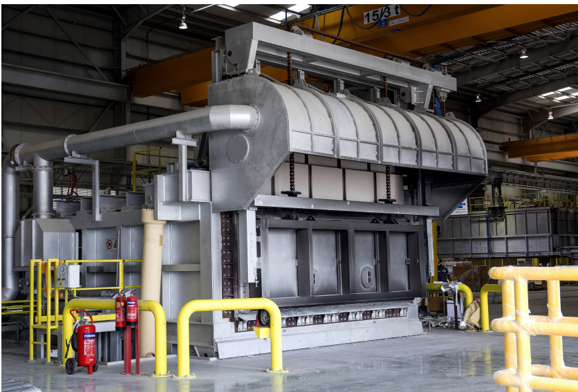
Casting Furnace, capacity 30 tonnes
