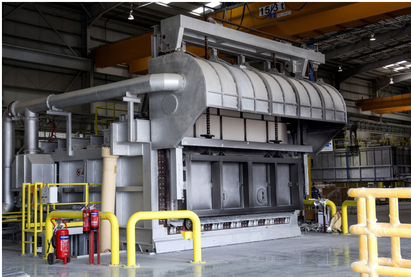
Casting Furnace, capacity 30 tonnes
