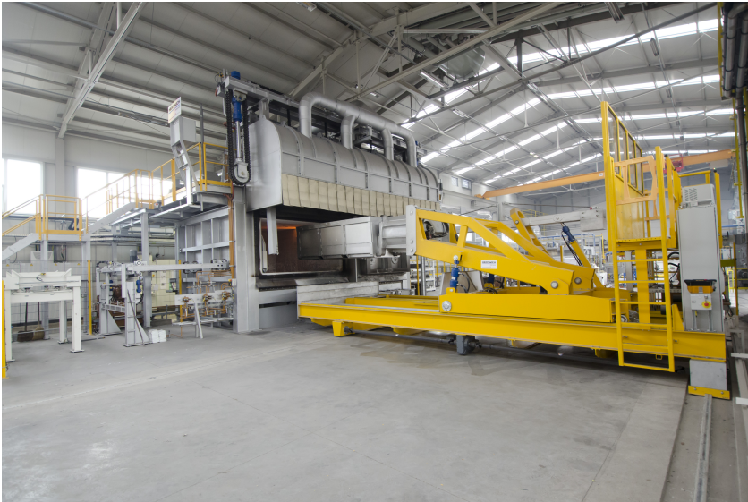
Hertwich Multi-Chamber Melting Furnace with preheat ramp (Ecomelt PR), similar plant
