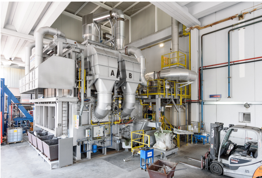
Hertwich chip melting furnace at Cromodora, Italy
